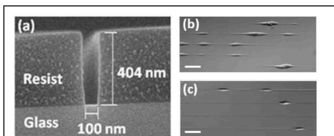
Fig. 1. (a) SEM image of cross section of the EB lithographed nano line pattern. (b,c) hbmMSC cultured on the line patterns of 500 nm width. (b) 100 nm depth and (c) 400 nm depth. Scale bar = 100  $\mu$ m.
