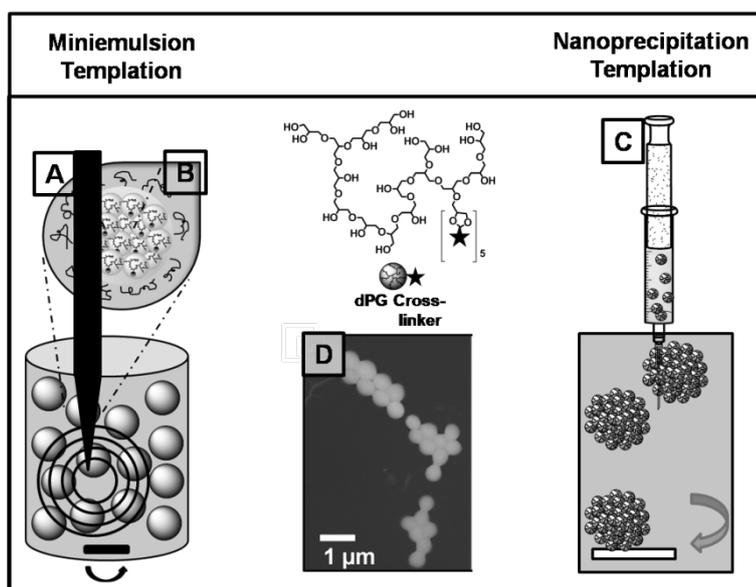
Figure 1. Schematic representation of nanogel preparation by miniemulsion templation using strong ultrasonication (A: black bar) and block-co-polymer surfactants (B: black lines), nanogel preparation by templation using surfactant and ultrasound free nanoprecipitation technique (C), transmission electron micrograph of the obtained nanogels by nanoprecipitation (D).
